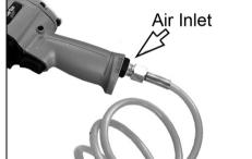
If using a mini oiler, place a sheet of paper next the exhaust port and hold the throttle open for approximately 30 seconds. The oil volume is correctly set when a light stain of oil can be seen on the paper. Excessive oil should be avoided.
