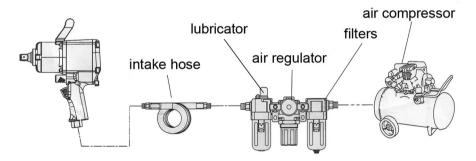
A typical airline layout is shown above. If an automatic in-line filter/regulator is used, it will keep the air tool in good condition, but should be regularly checked and topped up with oil. SAE 10 oil should be used and the lubricator adjusted to approx 2 drops per minute.
