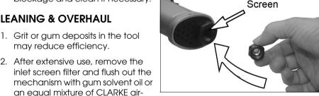
3. If the tool still runs erratically or becomes inefficient, and the air supply is of good quality, it may be necessary to dismantle the air motor and replace worn or damaged parts. You may prefer to take the tool to your CLARKE dealer if internal maintenance is required.
